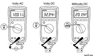
Figure 1. Measuring AC and DC Voltage
