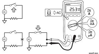
Figure 2. Measuring AC and DC Current
